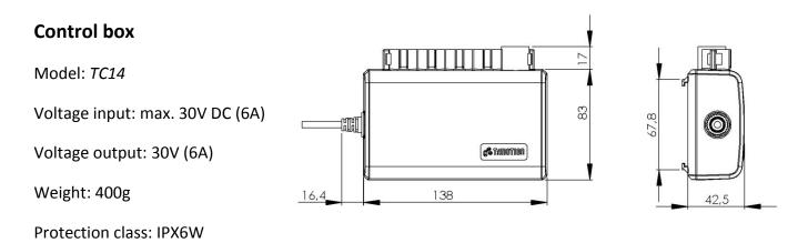
*Note:* The control box power supply cable is the main disconnect means.
